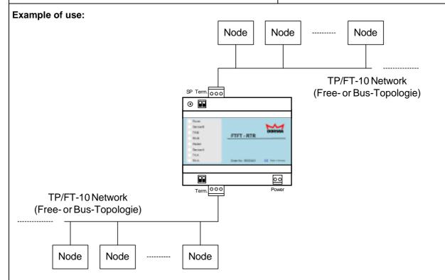
This router may be used to connect TP/FT-10 channels to support additional nodes or extend the maximum channel length. The two channels connected to a router are physically isolated, so a failure on one channel does not affect the other. To improve overall network performance, routers can be used to isolate traffic within subsystems
